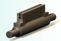
Two - Up Head: - Two Crimp / Jaws mounted on ech shaft.
